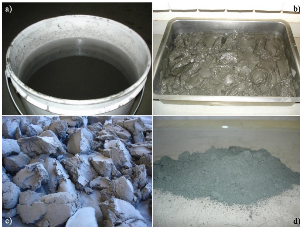
Figure 3. Tailings as received in the laboratory (a); after most of the water was removed (b); after drying in the oven (c); after breaking the clods (d).
